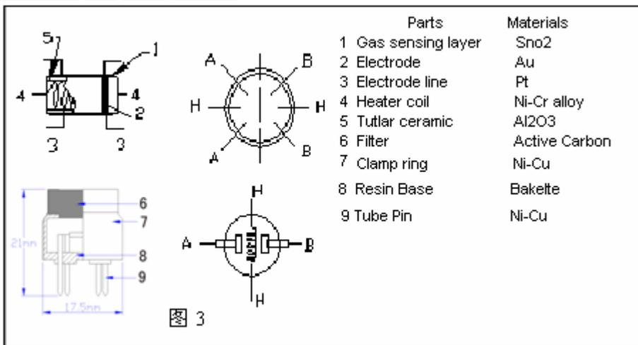
Structure and configuration of MQ-7 gas sensor is shown as Fig. 3, sensor composed by micro AL<sub>2</sub>O<sub>3</sub> ceramic tube, Tin Dioxide (SnO<sub>2</sub>) sensitive layer, measuring electrode and heater are fixed into a crust made by plastic and stainless steel net. The heater provides necessary work conditions for work of sensitive components. The enveloped MQ-7 have 6 pin, 4 of them are used to fetch signals, and other 2 are used for providing heating current.
