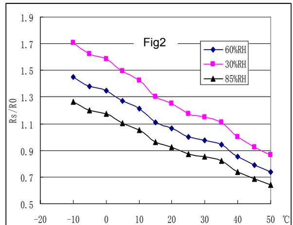
Fig.2 shows the typical temperature and humidity characteristics. Ordinate means resistance ratio of the sensor ( $R_s/R_0$ ),  $R_s$  means resistance of sensor in 100ppm CO under different tem. and humidity.  $R_0$  means resistance of the sensor in environment of 100ppm CO, 20°C/65%RH
