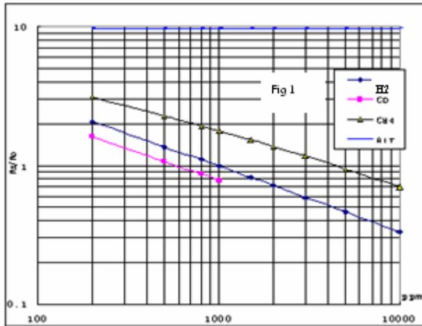
Fig.1 shows the typical sensitivity characteristics of the MQ-7, ordinate means resistance ratio of the sensor ( $R_s/R_0$ ), abscissa is concentration of gases.  $R_s$  means resistance in different gases,  $R_0$  means resistance of sensor in 1000ppm Hydrogen. All test are under standard test conditions.
